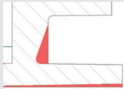
optimisation by reducing material in corners
