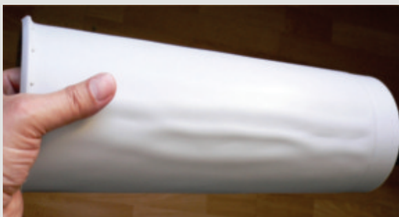
volume contraction of non-reinforced polypropylene (PP) can be up to 20%
